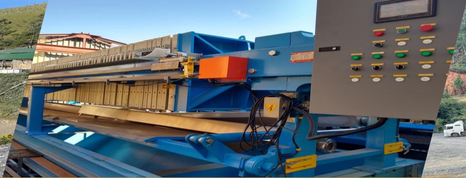
Filter Press to extract water from the concentrate
